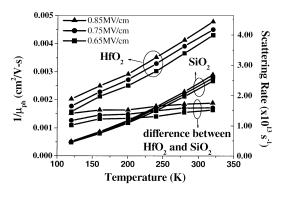
Fig. 4. Scattering rate due to phonons for nMOSFET with  $HfO_2$  or  $SiO_2$  as gate dielectric, indicating additional scattering in the  $HfO_2$  sample as compare to the  $SiO_2$  sample. The difference between the two is also plotted, and is attributed to scattering by soft optical phonons in  $HfO_2$ .
