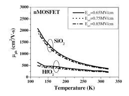
Fig. 3. Mobility limited by phonon scattering,  $\mu_{\rm ph}$ , for nMOSFET with HfO<sub>2</sub> or SiO<sub>2</sub> as gate dielectric at various effective electric fields from 0.65 mV/cm to 0.85 MV/cm.
