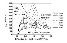
Fig. 1. Effective electron mobility in HfO<sub>2</sub>-gated nMOSFET at various temperatures from 120 to 320 K, with and without interface-trap correction, as compared to universal mobility over the same temperature range.
